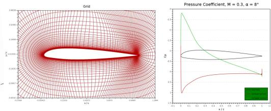
C81Gen provides a table of lift, drag, and moment coefficients in C81 format based on user-specified Mach numbers and angles of attack.
