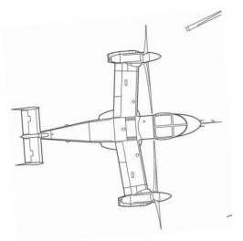
A tiltrotor configuration utilizes rotors that are capable of rotating to either produce vertical left or horizontal thrust. These configurations typically consist of two rotors near the ends of a fixed wing.
