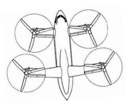
The Bell Boeing Quad Tilt Rotor (QTR) is a variation on the standard tiltrotor design. This configuration, which is designed for large payloads, utilizes four rotors that are able to rotate about a nacelle.
